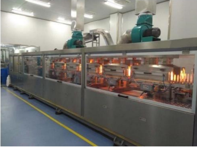
ISBM line installed by SQH for Mediflow Pakistan.
