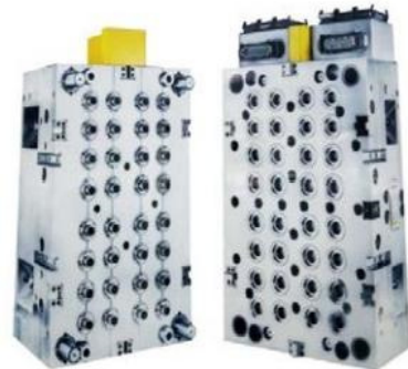
Mold for Euro-caps (From 8-96cavities)
